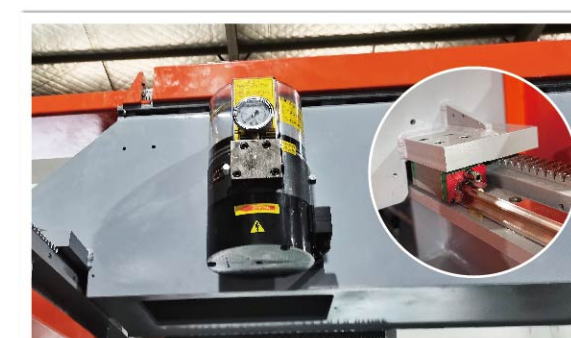
6.润滑系统和线性导轨，保证机械的精度和耐用度 Lubrication system and linear guide rail to ensure the accuracy and durability of machinery.
