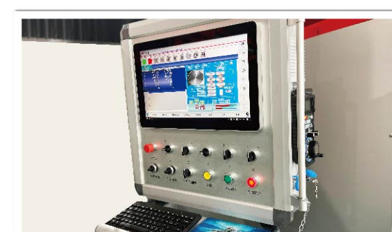
8.意大利的控制系统，有避免碰撞和管理生产订单的功能 Italian control system can prevent collision also can managing production
