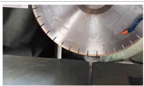
1.自动测量锯片直径和工具高度 Automatically measure the diameter of disk and length of tools
