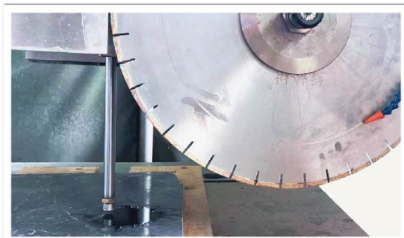
2.自动测量板材厚度 Automatic measurement of slab thickness
